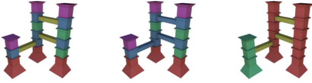
Figure 12: Left: A model is decomposed manually in 18 pieces of 5 types. Middle: The optimized version consists of 12 pieces of 4 types. Right: Allowing replacement of approximately matching tiles further reduces the complexity to 6 pieces of 3 types.
