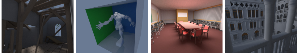
Figure 3.2: Four examples of diffuse path tracing with 300 paths per pixel. From left to right - Ruins, Ogre, Conference and Venice
