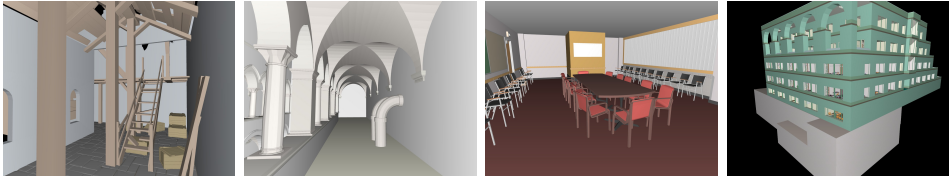
Figure 4.3: Some of our test scenes, from left to right - Ruins, Sponza, Conference, and Soda Hall. We can render these viewpoints at 25, 43, 11 and 8 fps with simple shading in a 1024 \times 1024 window and can construct grids in 10, 13, 27 and 130 milliseconds on a GTX280.
